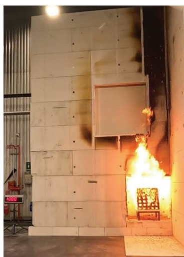
Figures 4 and 5: Façade fire test set-ups for EU research project on an inert façade (large and medium exposure) [5]
