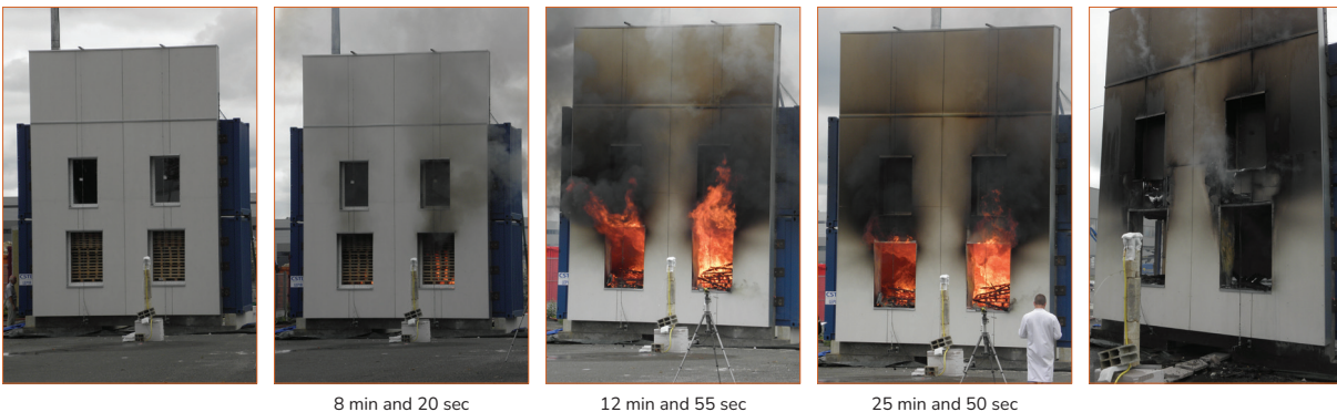
Figure 11: Photos illustrating the test stages of the LEPIR 2 test on a façade with PIR insulation
