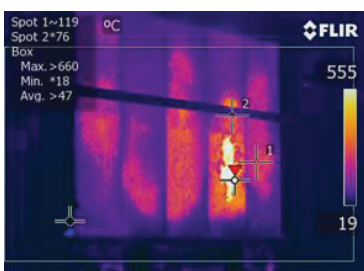
Figure 22 (above): Test build-up according to EN 1365-1: the unexposed face of the specimen
