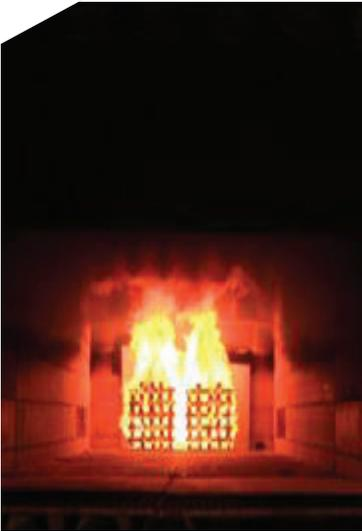
Figure 2: Steel deck flat roof test according to DIN 18234-1:2003-09 in Germany
