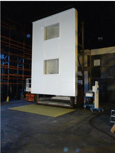
Figure 4: Fire façade test set up according to NFPA 285
