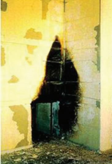
Figure 3: Damage of the test sample: PU insulation layer
