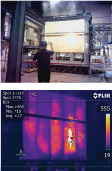
Figure 9: Test build-up according to EN 1365-1: the unexposed face of the specimen and thermographic image during test
