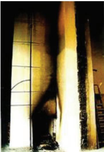
Figure 2: Damage of the test sample: render finishing
