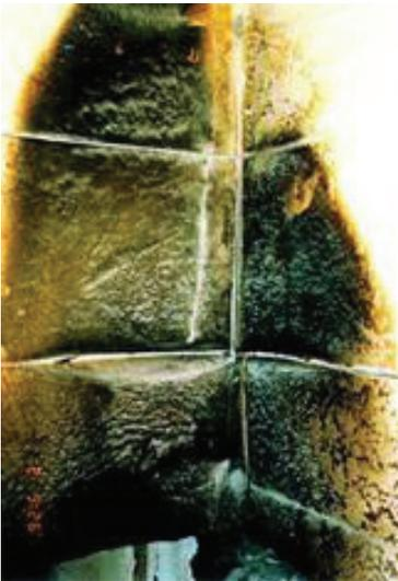
Figure 4: Damage of the test sample: fire room
