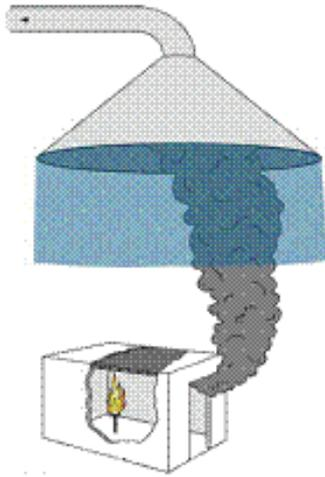
Figure 5: Schematic drawing of the test set-up under a large calorimeter hood
