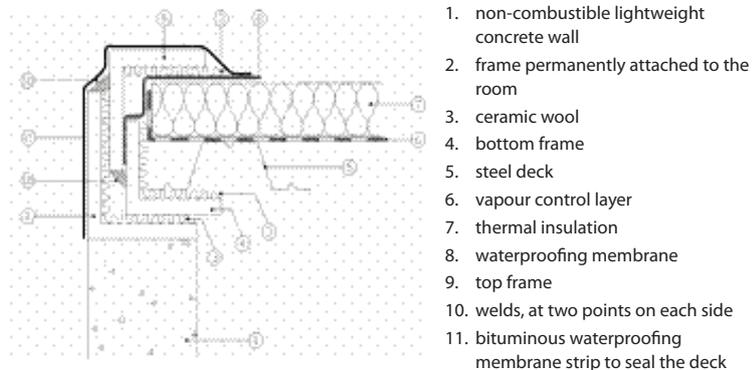
The complete roof assembly was mounted in a closed frame on top of the test room. The frame is set at a slope of 2%, with the lower side above the back wall. The channels in the steel deck are laid parallel to the length of the building. The thickness of insulation material is varied according to its declared thermal conductivity so as to achieve the same R-value.
