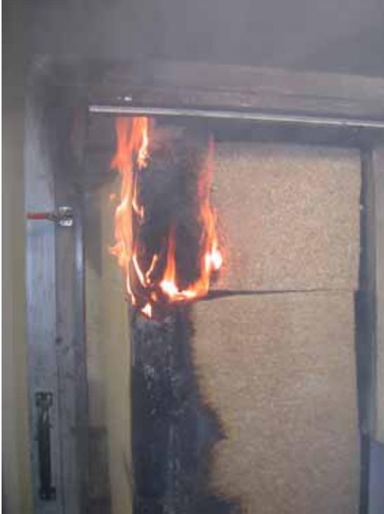
Self-ignition after test while removing sample from SBI
