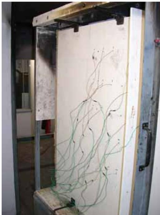
Thermocouples and substrate board
