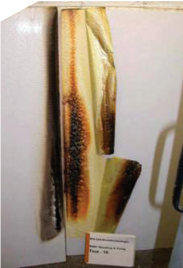
Figure 4: PU board with gypsum (plasterboard) cover achieving class B in SBI test according to EN 13823
