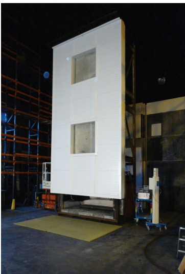
Figure 6: Façade fire test set up according to NFPA 285
